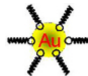
Figure 1: Gold nanoparticles with attached thiol chains.
