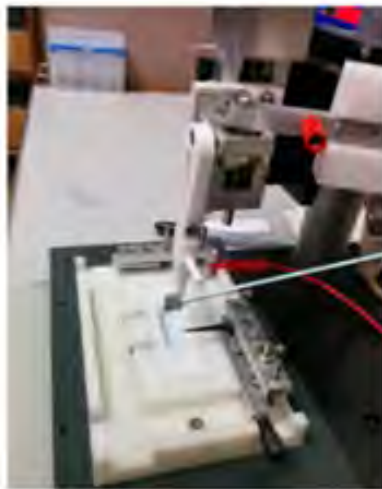
Fig. 1: (left) Apparatus for dip-coating (“combing”) DNA molecules onto a substrate by withdrawal from solution. (right) Schematic of stretching and straightening of DNA on the surface by preferential end adsorption
